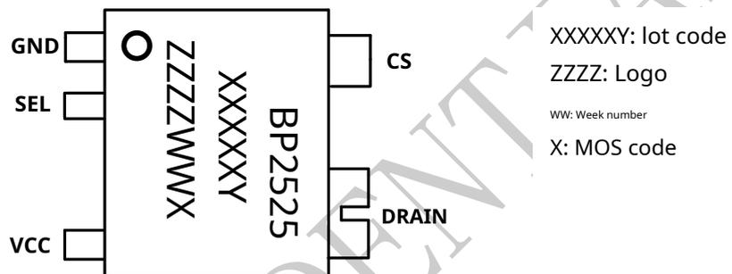
Figure 2 Pin package diagram
