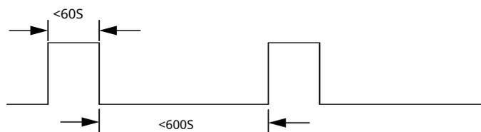
picture 3 Schematic diagram of instantaneous pulse
