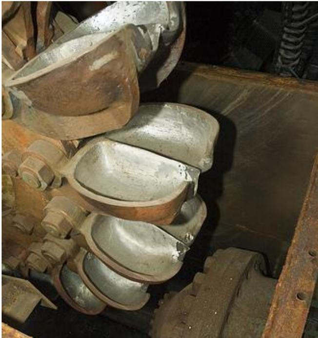
Fig 5. Buckets on the "A" Pelton wheel at Boulder Canyon Hydroelectric facility.
